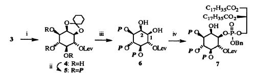
i. n-Bu<sub>4</sub>NF·H<sub>2</sub>O, PhCO<sub>2</sub>H (85%); ii. (PhCH<sub>2</sub>O)<sub>2</sub>PN<sup>t</sup>Pr<sub>2</sub>, 1*H*-tetrazole, then mCPBA (72%); iii. CF<sub>3</sub>CO<sub>2</sub>H, commercial CH<sub>2</sub>Cl<sub>2</sub> (83%); iv. dibenzyl 1,2-distearoyl-sn-glyceryl phosphite, Py HBr<sub>3</sub>, 2,6-dimethylpyridine (36%). Abbreviations: Lev=CH<sub>3</sub>CO(CH<sub>2</sub>)<sub>2</sub>CO;  $P = (BnO)_2P(O)$ ; Bn=benzyl; Py=pyridine
